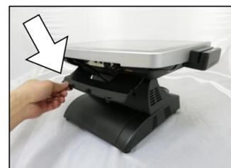
4. Push down IO cover to access IO ports.
