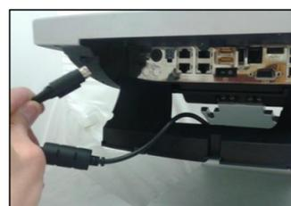
4. Connect power to IO port. Connect other cables as needed.
