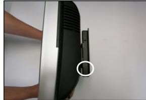
6. Secure machine to wall by installing M3x6mm screw. One on each side.
