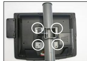
3. Secure the VESA 100 holes with four (4) M4x8mm screws.
