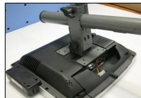
2. Align pole mount with back bezel of machine.
