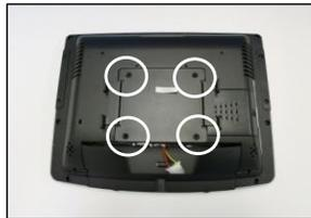
3. Secure plate with four (4) M4x8mm screws.
