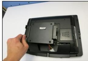
2. Align smaller piece of wall mount plate with recess on back of machine.
