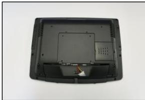
1. Place machine face down on a clean & flat surface.
