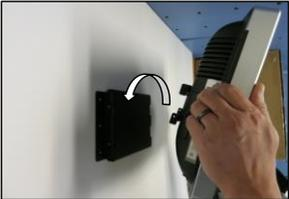
5. Align the hook from machine with slot on wall mount plate & slide in to latch.
