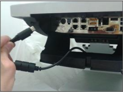
4. Connect power to IO port. Connect other cables as needed.
