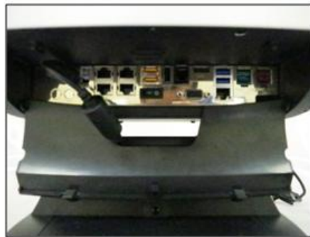
5. Route cables to the front and connects them to respective ports. And close lid when done.
