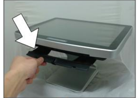
3. Push down IO cover to access IO ports.
