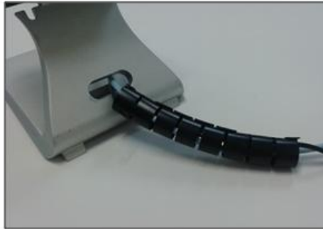
5. Organize cables using cable tube included in the package.
