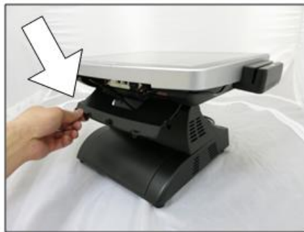
4. Push down IO cover to access IO ports.
