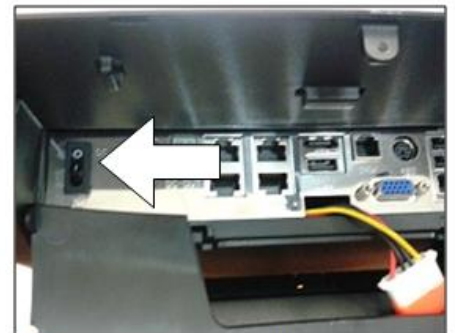
6. Toggle power switch to turn on terminal.
