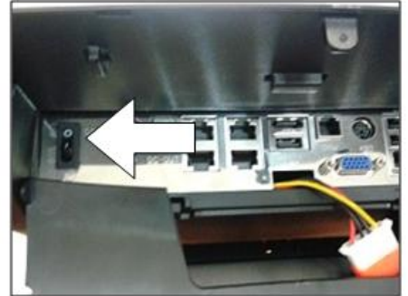
6. Toggle power switch to turn on terminal.
