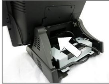
2. Route cables of peripherals through opening.
