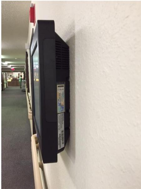
6.) FASTEN KIOSK TO WALL MOUNT PLATE WITH 4 SCREWS (Small Black Screws Provided)
